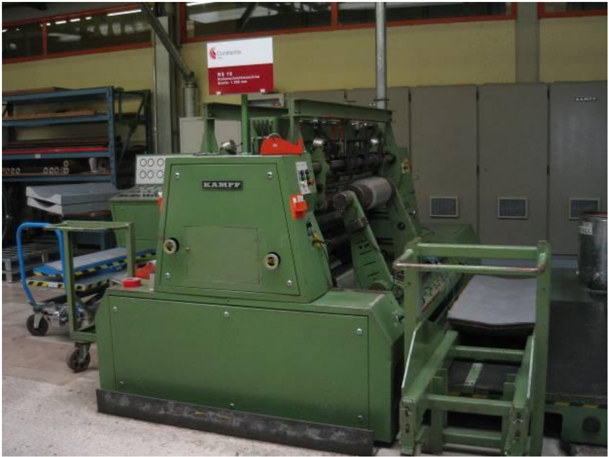
Finished reel unloading carriage
